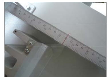
▲ manual backgauge with measuring scale, scale with mm/inch(430M/480M)
