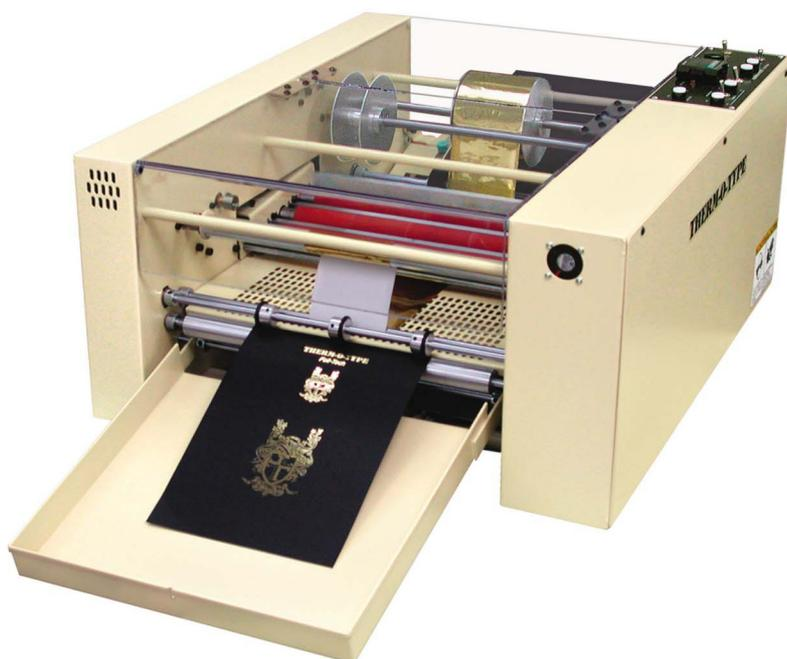
**“Foil Fusing”** or **“Sublimation Foiling”** is the method of bonding foil to a toner image printed by a copier machine or laser printer. Using Foil-Tech equipment, customers can now efficiently produce a wide range of high value products. Sheets up to 370mm (14½”) wide by 610mm (24”) long can be run through the machine.
